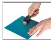
step 1: make grid cutting on surface
