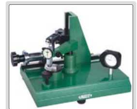
Test the effect of lateral force on accuracy of test indicators (half round gage block is required)
