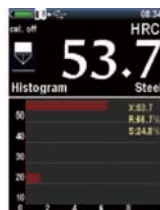
Histogram display mode, show average value, relative range and relative standard deviation
