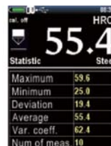
Statistics display mode, show maximum, minimum, deviation, average, relative range and test times
